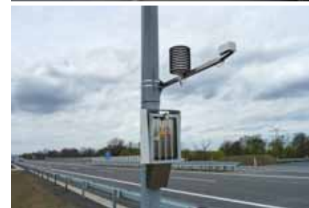
Road Weather CrossMet, METIS Czech Republic, highways, motorways and 1st class roads
